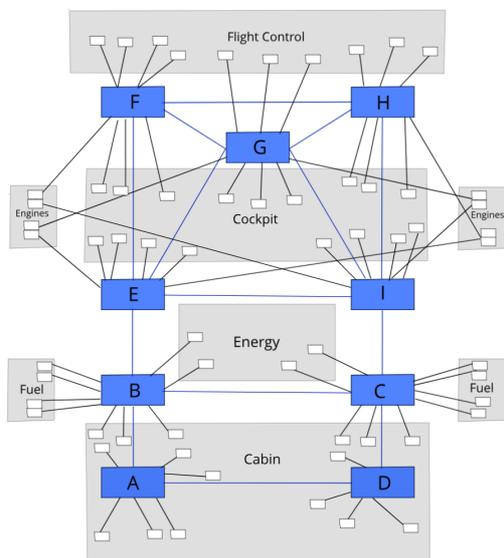
Figure 1: Structure of AFDX on the A380
