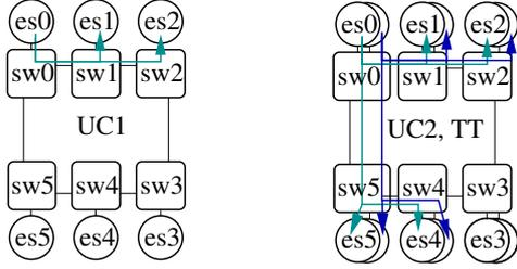
**Figure 4: Illustration of 1 VL of each end-system connected to switch  $sw_0$ , with  $N=6$  and  $L=2$ , for use-cases  $UC_1$ ,  $UC_2$  and TT traffic.**
