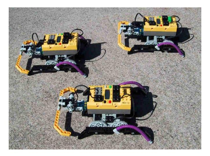
swarms of robots, Hitachi H8 microcontroller 16MHz, IR link
